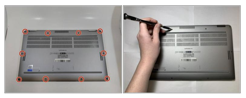
Use a Phillips #00 screwdriver to loosen the ten captive screws.
