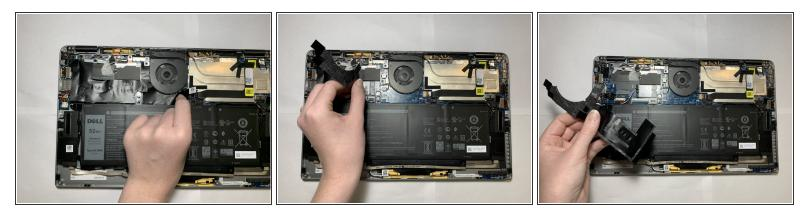
• Carefully peel back and remove the black tape around the top left corner of the motherboard.
