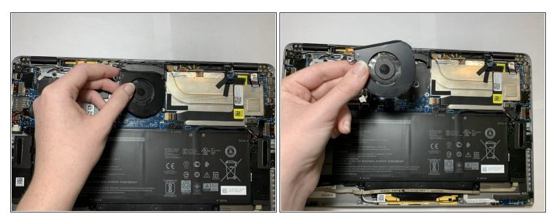
• Lift the fan up and out.
