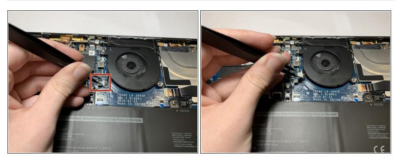
• Grip both sides of the fan connector plug with tweezers, and pull directly backwards, toward the cables, until the plug disconnects.
