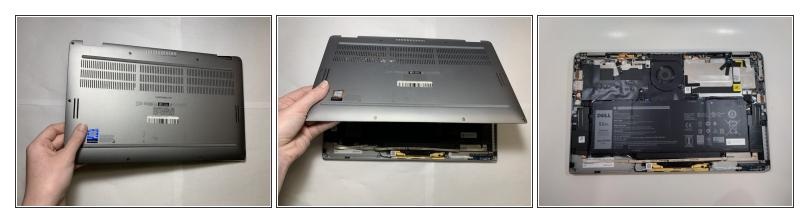
• Carefully lift off the back panel.
