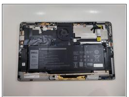
Carefully lift off the back panel.
