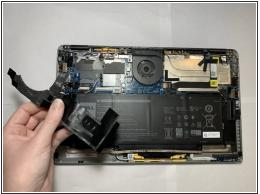
Carefully peel back and remove the black tape around the top left corner of the motherboard.
