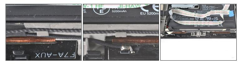
• Fit the speaker cable into the two hooks along the bottom of the chassis.
