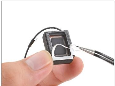
• Peel off and discard the liners on the speakers themselves, exposing the adhesive underneath.
