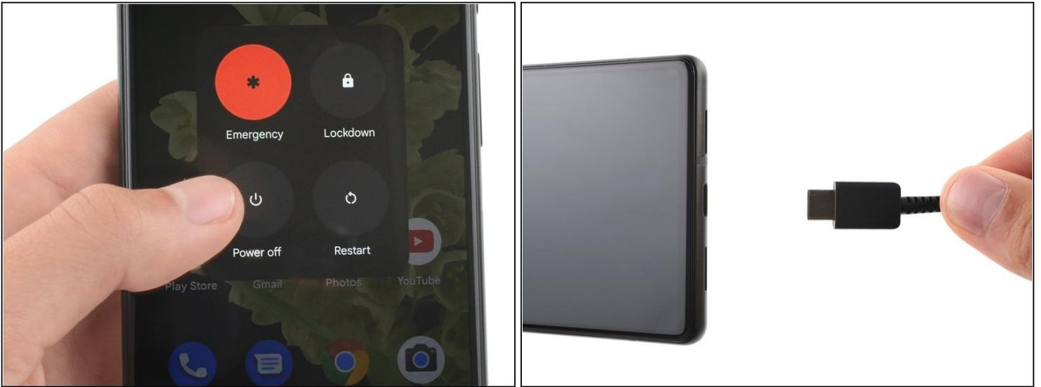
**⚠️ Allow your battery to drain below 25% before starting this repair. A charged battery may catch fire if damaged.**
