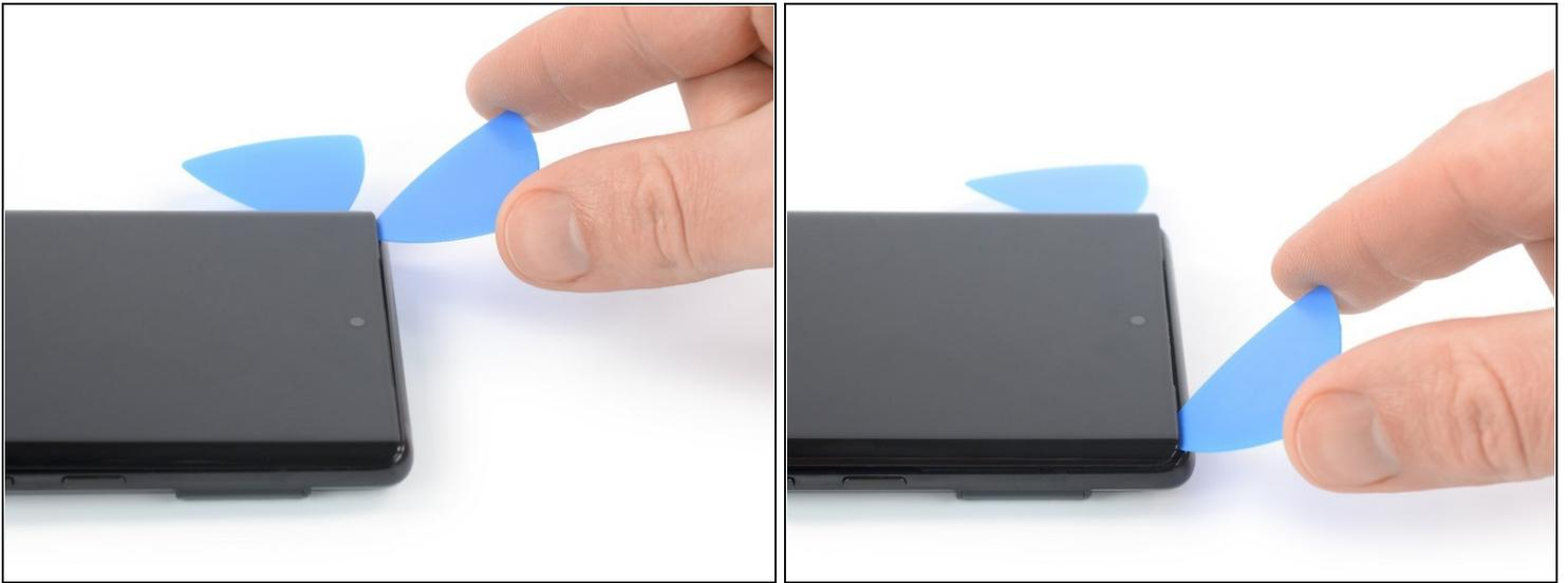
ⓘ If the adhesive becomes hard to cut, it has most likely cooled down. [Use your iOpener](#) or heat gun for 1-2 minutes to reheat it.
