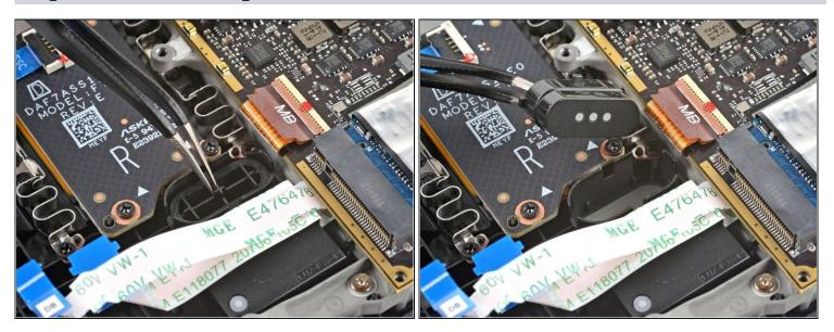
• Use a pair of tweezers to remove the quick access button.
