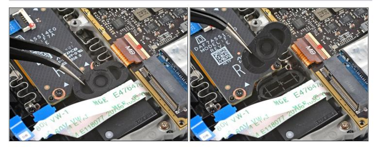
• Use a pair of tweezers to remove the quick access button membrane.
