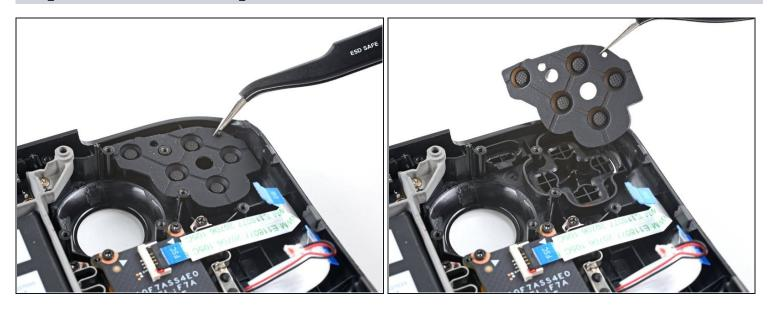
• Use a pair of tweezers to remove the D-pad membrane.
