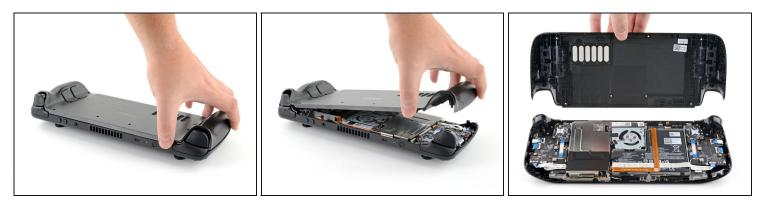
(i) Once the clips are disconnected from one edge, the rest disconnect easily.
