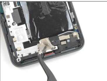
Use a spudger or a pair of tweezers to peel back the tape securing the charging port bracket to the speaker assembly.
