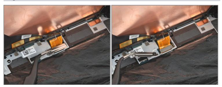
• Use a pair of <u>tweezers</u> to remove the screen connector bracket.
