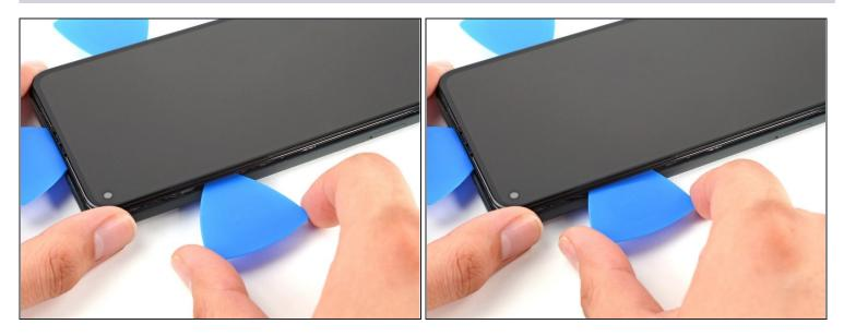
• Insert the tip of an opening pick into the *bezel seam* about 3-4 cm below the front-facing camera.
