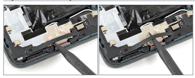
Use the pointed end of a spudger to pry up on the black plastic cover at the bottom left of the phone.
