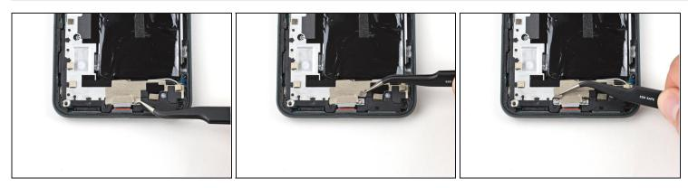
• Use a pair of <u>tweezers</u> to slightly peel back the tape concealing the two screws securing the charging port bracket.
