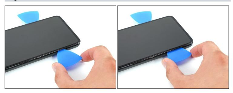
• Insert the tip of an opening pick into the *bezel seam* on the left side of the phone, about 2 cm from the bottom of the phone.
