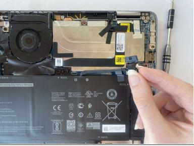
• Grip the battery cable near the plug and pull it straight out, in the direction of the cable.
