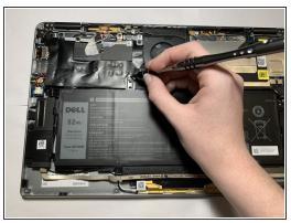
• Use a Philips #00 screwdriver to remove one 4.5 mm screw.
