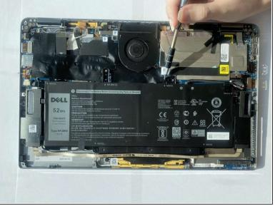
• Use a Philips #00 screwdriver to remove the five 3mm screws that secure the battery.
