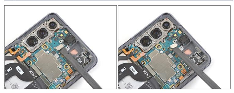
• Use the flat end of a spudger to pry up and disconnect the front camera's press connector.
