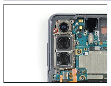
Use a Phillips screwdriver to remove the 4 mm screw securing the camera bracket and the motherboard to the frame.
