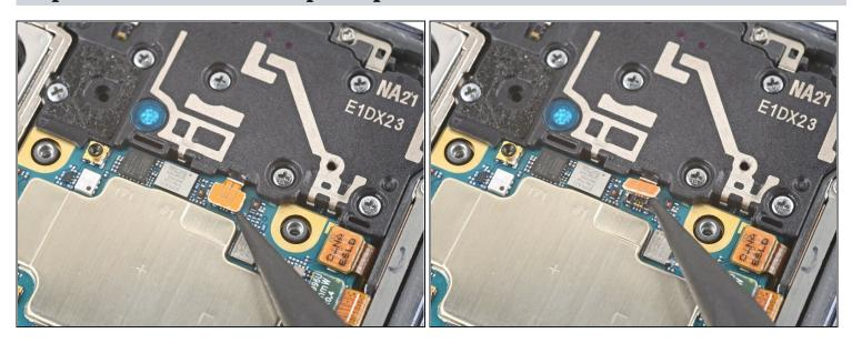
• Use the point of a spudger to pry up and disconnect the earpiece speaker cable's press connector.
