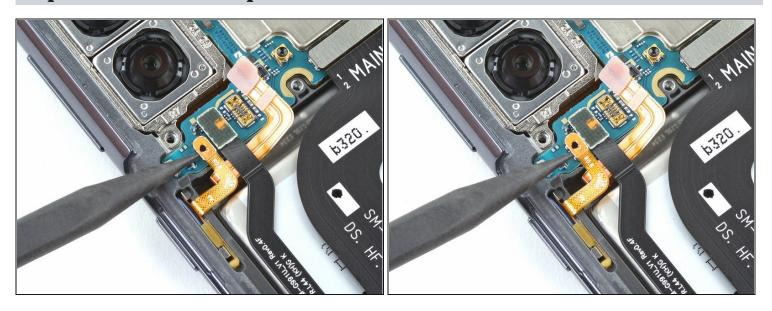
• Use the point of a spudger to pry up and disconnect the power button cable's press connector.
