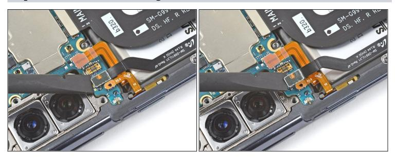
Use a spudger to pry up and disconnect the 5G antenna cable's press connector.
