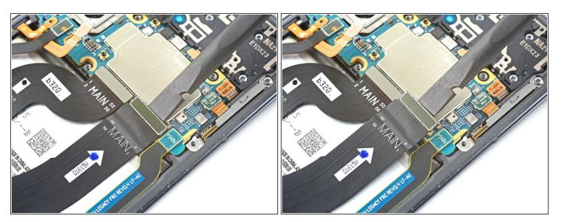
Use the flat end of a spudger to pry up and disconnect the primary interconnect cable's top press connector.
