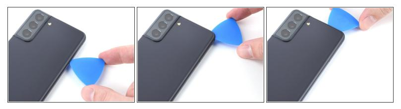
• Rotate the right-edge opening pick around the top-right corner of the phone.
