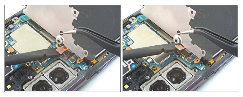
While using tweezers, or your fingers, to hold the motherboard bracket out of the way, use a spudger to pry up the battery press connector.
