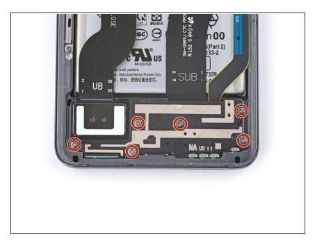
Use a Phillips screwdriver to remove the six 4 mm screws securing the loudspeaker to the frame.
