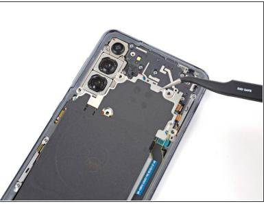
• Use a pair of tweezers to gently pull up and unclip the motherboard bracket from the frame.
