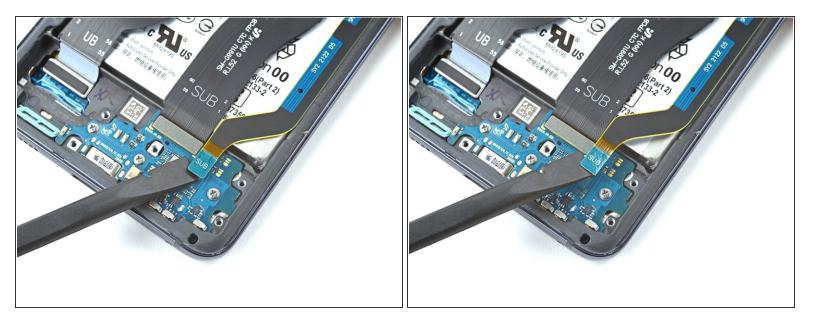
Use the flat end of a spudger to pry up and disconnect the secondary interconnect cable's bottom press connector.
