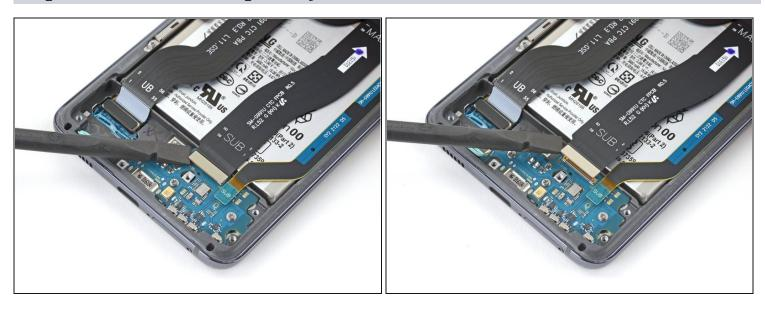
• Use the flat end of a spudger to pry up and disconnect the primary interconnect cable's press connector.
