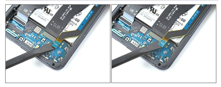
• Use the flat end of a spudger to pry up and disconnect the secondary interconnect cable's press connector.
