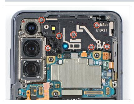
Use a Phillips screwdriver to remove the seven 4 mm screws securing the earpiece speaker to the motherboard.
