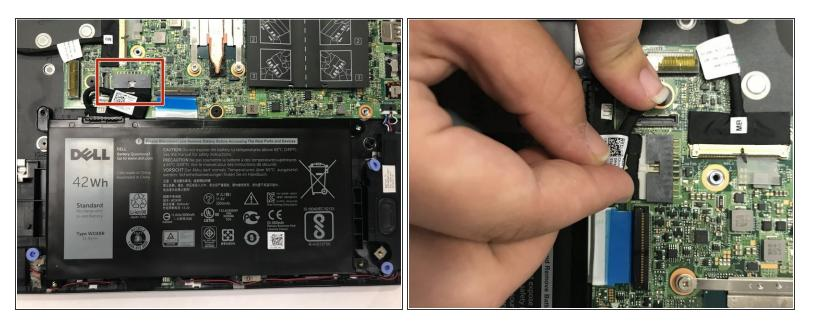
Disconnect the battery's black connector from the motherboard.
