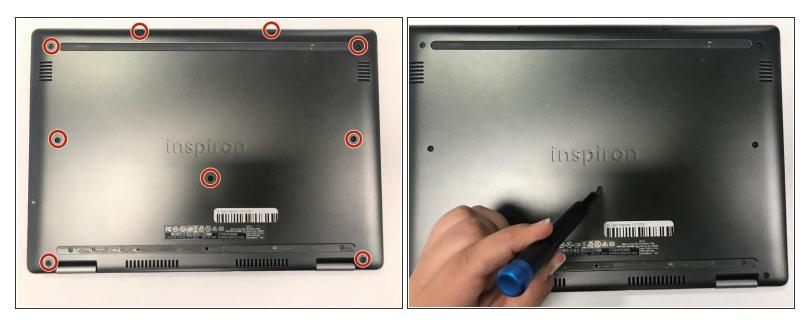
Using a Phillips #00 screwdriver, extract the nine 3 mm screws located on the back of the laptop.
