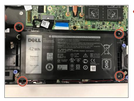
Remove the four screws from the battery using a Phillips #00 screwdriver.
