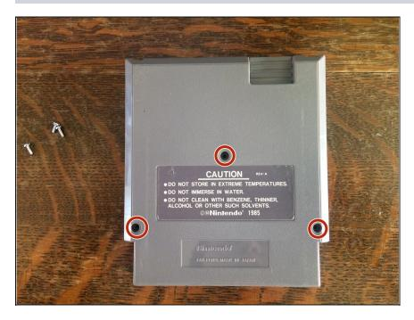
Use a 3.8 mm gamebit screwdriver to undo the 3 screws on the rear of the cartridge, and set them aside.
