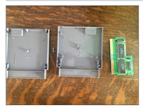
• Gently lift out the PCB, and clean the pins with isopropyl alcohol and a cotton swab. if the pins still remain dirty, carefully sand the pins with a very fine-grit sandpaper.
