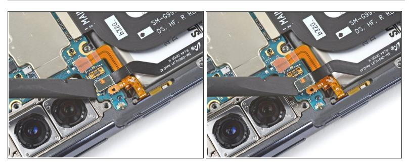
• Use the flat end of a spudger to pry up and disconnect the 5G antenna cable's press connector.
