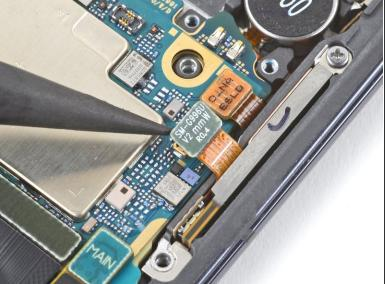
Use a spudger to pry up and disconnect the 5G antenna cable's press connector.
