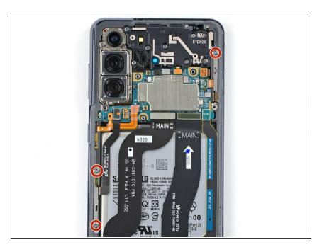
Use a Phillips screwdriver to remove the three 3.5 mm screws securing the 5G antenna brackets to the frame.
