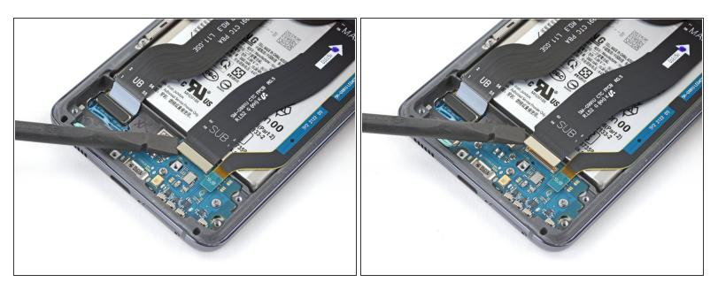
Use the flat end of a spudger to pry up and disconnect the primary interconnect cable's bottom press connector.
