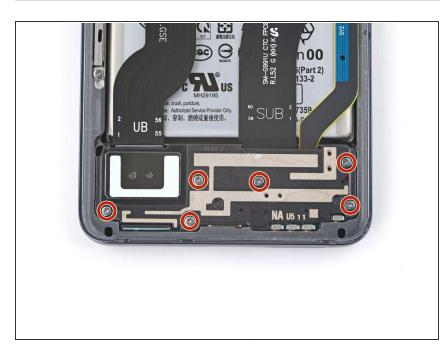
Use a Phillips screwdriver to remove the six 4 mm screws securing the loudspeaker to the frame.
