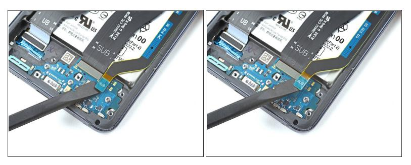
Use the flat end of a spudger to pry up and disconnect the secondary interconnect cable's bottom press connector.
