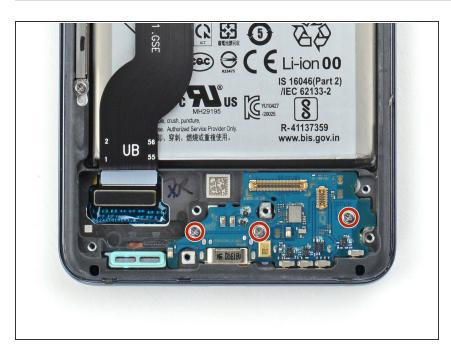
• Use a Phillips screwdriver to remove the three 3.5 mm screws securing the daughterboard to the frame.
