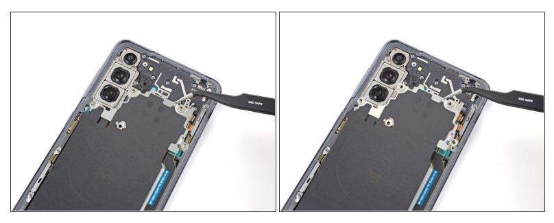
• Use a pair of tweezers to gently pull up and unclip the motherboard bracket from the frame.
