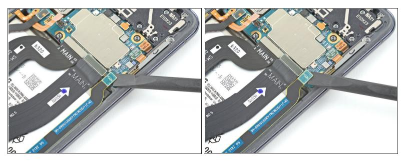
Use the flat end of a spudger to pry up and disconnect the secondary interconnect cable's top press connector.
