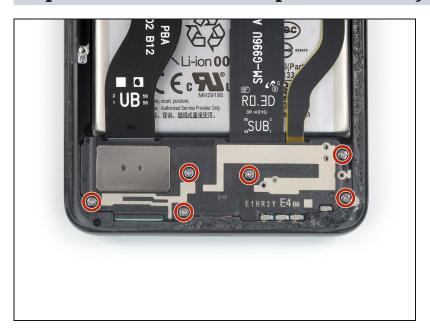
Use a Phillips screwdriver to remove the six 3.9 mm-long screws securing the loudspeaker assembly.
