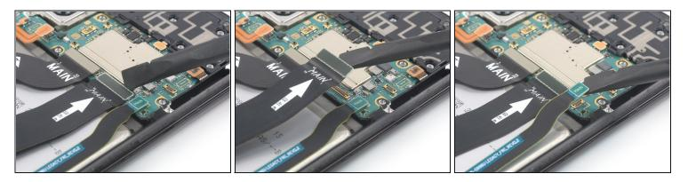
• Use a spudger to disconnect the main and interconnect flex cables from the motherboard by prying their upper connectors straight up from their sockets.
