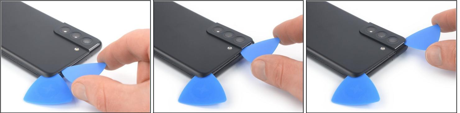
**⚠** When you slice near the camera assembly, insert only the tip of the opening pick (~4-5 mm) to avoid damaging or smearing the camera.
