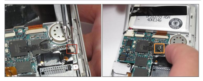
• Use <u>tweezers</u> to unplug the speaker wire from the motherboard by pulling the plug (not the wires) down towards the speaker.
