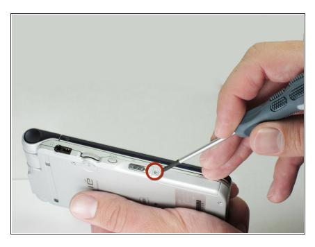
Unscrew the 2.5mm screw located on the left side of the device with a Phillips #00 screwdriver.
