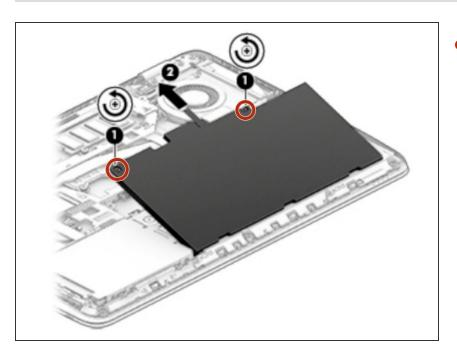
Loosen the two captive screws and remove the battery from the computer
