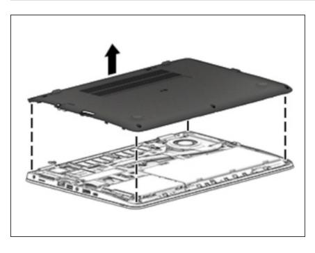
Pry up on the top (near the display hinge) of the bottom cover to disengage it from the computer.
