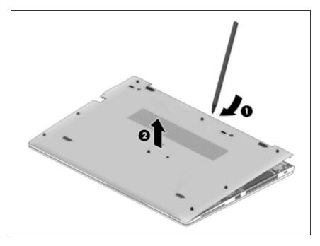
Starting under the middle of the display, pry and lift the bottom cover off the computer. Consider using a spudger.
