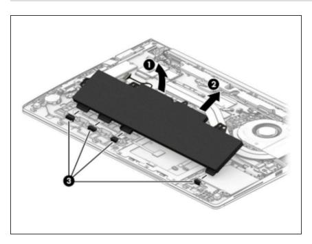
Rotate the top of the battery upward, and then lift the battery out of the computer.
