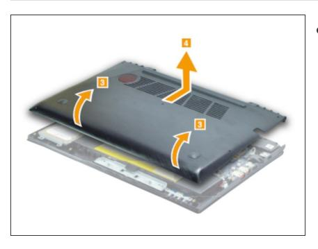
Remove the base cover in the directions shown by arrows.
