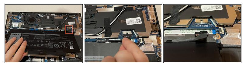
A Be careful not to break the connector by pulling too hard on the black tab.
