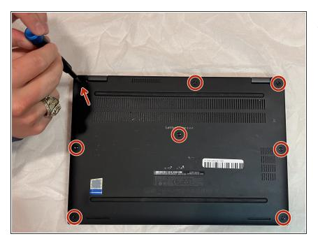
Using your Phillips #1 screwdriver, remove the eight 6 mm screws around the border of the bottom panel.
