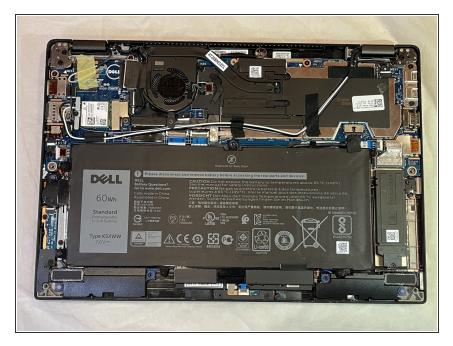
• Finally, lift the back panel off to uncover the inside of your Dell Latitude 7390.
