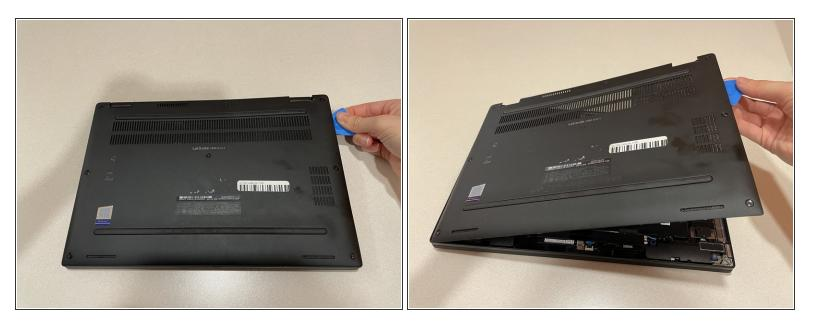
• Using an opening tool or picks, work your way around the periphery and pry the back case off.
