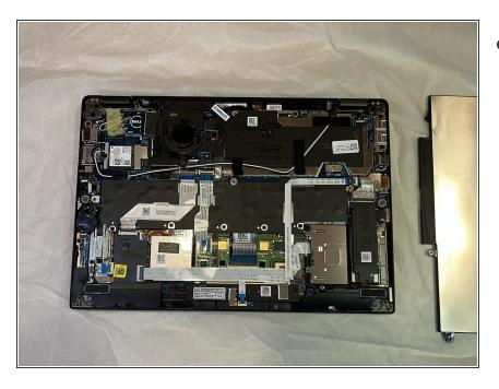
• Carefully lift the battery out of the laptop.
