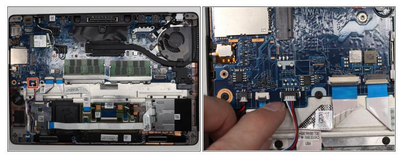
• Unplug the four pin speaker connector from the motherboard.
