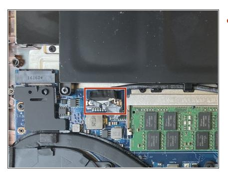
Use the pull tab on the battery connector to lift the connector straight up off its socket on the motherboard, disconnecting it.
