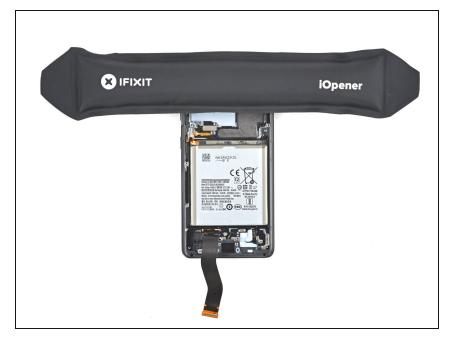
Apply a heated iOpener to the front camera for 90 seconds.
