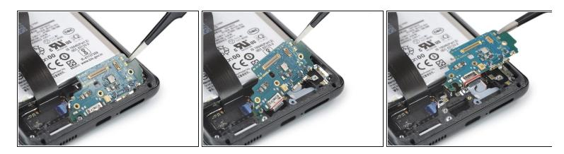
Use a pair of blunt tweezers or your fingers to remove the charging board. Start by lifting its top edge up and then carefully slide the USB-C connector out of its recess.
