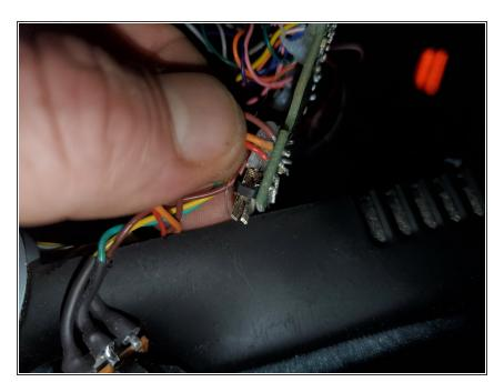
trigger switch wires(desoldering to make this easier)
