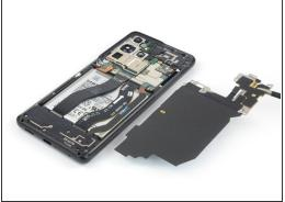
Use a pair of tweezers or your fingers to carefully remove the NFC antenna and charging coil assembly.
