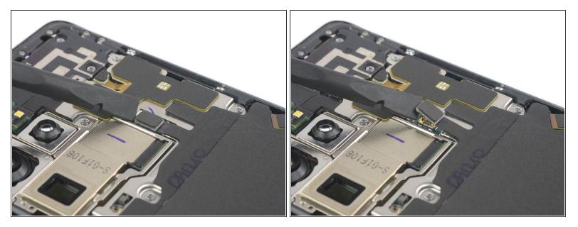
• Use a spudger to disconnect the charging coil by prying the connector straight up from its socket.
