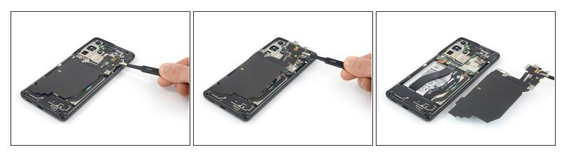
• Use a pair of tweezers or your fingers to carefully remove the NFC antenna and charging coil assembly.
