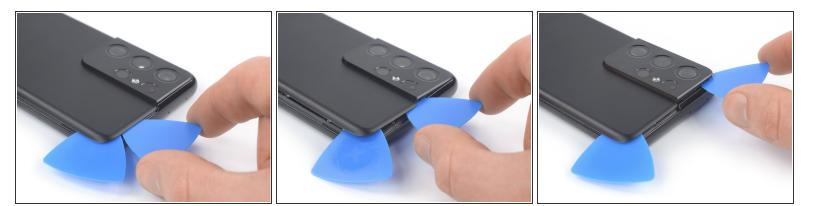
Men you slice near the camera assembly, insert only the tip of the opening pick (~ 4-5 mm) to avoid damaging or smearing the camera.
