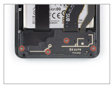
Use a Phillips screwdriver to remove the four 3.9 mm-long screws securing the loudspeaker assembly.
