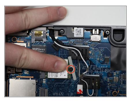
Remove the single screw from the Wi-Fi card using a Phillips #0 screwdriver.
