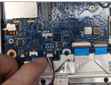
Unplug the four pin speaker connector from the motherboard.
