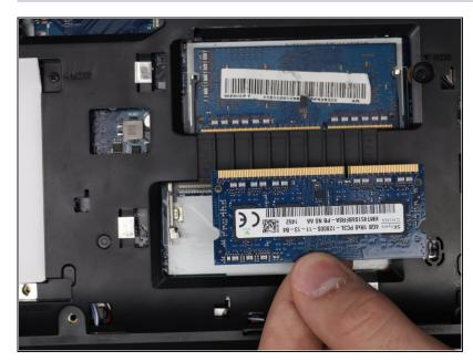
• Use your fingers to carefully remove the RAM chip by sliding it out at a ~45° angle.
