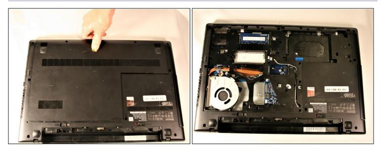
• Slide the cover away from the hinges and lift the panel off.
