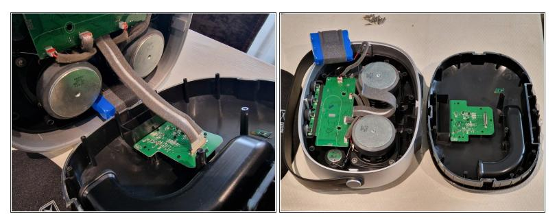
After you remove the 13 screws, put your finger in the woofer hole on the back of the speaker. Pull
