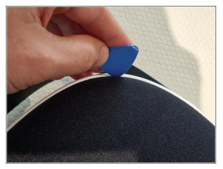
Use a pick to gently pull the cover. There are no fragile parts. The cover is made of metal and covered with a type of mesh.
