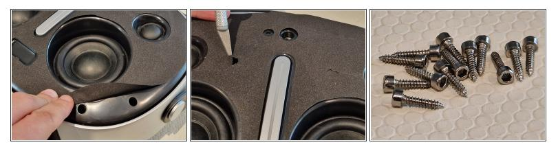
• Once the front cover is removed gently lift the thin protection layer in order to find the holes where the screws are located. In order to find the two middle screws you will have to make two small incisions as shown in the picture.
