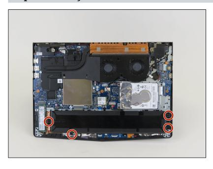
Remove the four 4 mm Phillips #00 screws securing the battery.
