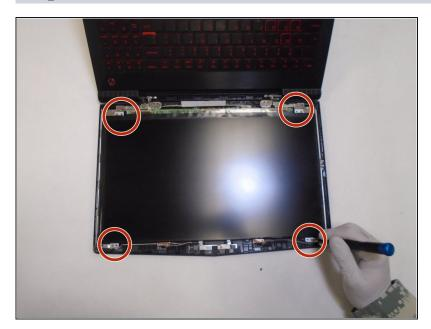
Remove the four 4 mm screws with a Phillips #1 screwdriver.
