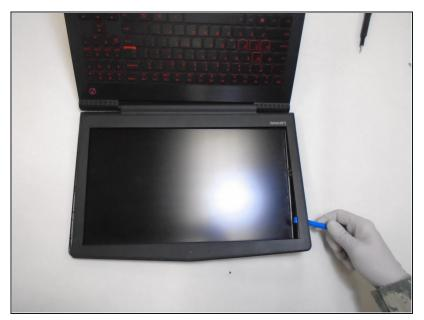
• Use an opening tool to pry off the display bezel.
