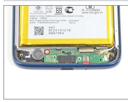
Use a T5 Torx screwdriver to remove the 3 mm screw securing the daughterboard to the midframe.
