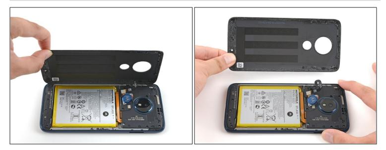
• Remove the rear cover, taking care not to damage the fingerprint sensor.
