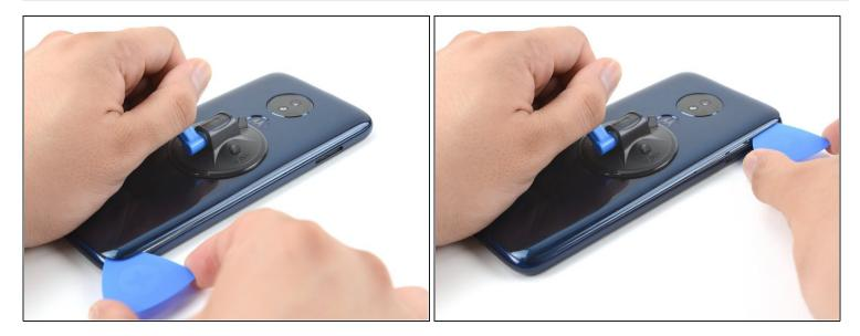
• Slide the pick along the gap on the same side of the phone as the SIM card tray to slice through the adhesive securing the rear cover to the midframe.
