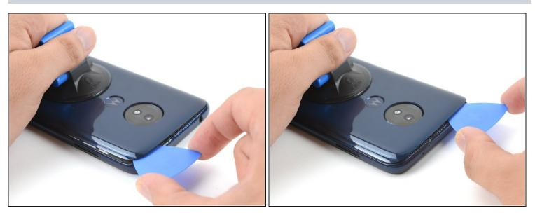
• Slide the pick along the gap at the top of the phone to slice through the adhesive securing the rear cover to the midframe.
