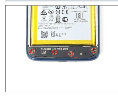
Use a T5 Torx screwdriver to remove the four 2.5 mm screws securing the daughterboard cover to the midframe.
