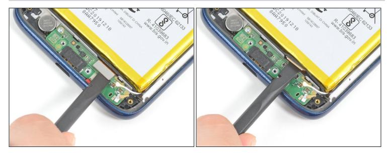
• Use the flat end of a spudger to pry up on the interconnect cable connector to disconnect it.
