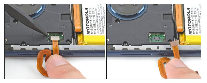
• Use the pointed end of a spudger to pry up on the fingerprint sensor connector to disconnect it.
