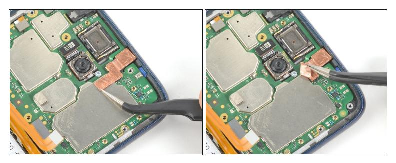
• Use a pair of tweezers to gently peel back the bottom of the copper sheet covering the metal shield below the front-facing camera.
