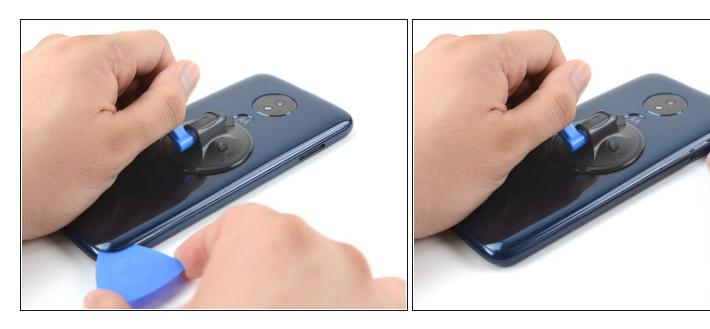
Slide the pick along the gap on the same side of the phone as the SIM card tray to slice through the adhesive securing the rear cover to the midframe.
