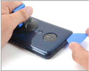
• Slide the pick along the gap at the top of the phone to slice through the adhesive securing the rear cover to the midframe.
