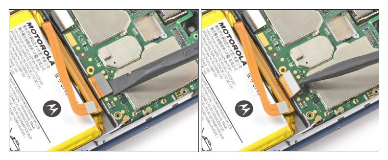
• Use the flat end of a spudger to pry up on the interconnect cable connector to disconnect it.
