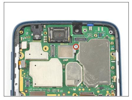
Use a T5 Torx screwdriver to remove the 3 mm screw securing the motherboard to the midframe.
