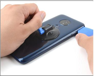
Slide the pick along the gap on the same side of the phone as the SIM card tray to slice through the adhesive securing the rear cover to the midframe.
