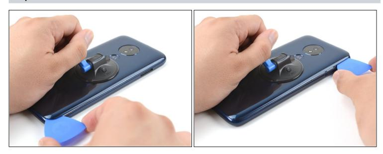
Slide the pick along the gap on the same side of the phone as the SIM card tray to slice through the adhesive securing the rear cover to the midframe.
