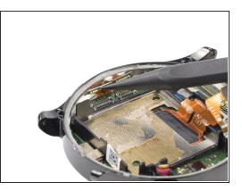
Use the tip of a spudger to pry up and disconnect both display cables.
