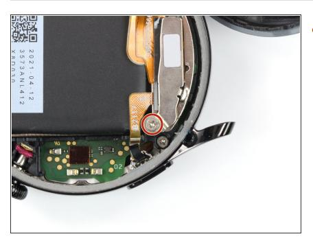
Use a Phillips screwdriver to remove the 2.9 mm-long screw from the sensor bracket.
