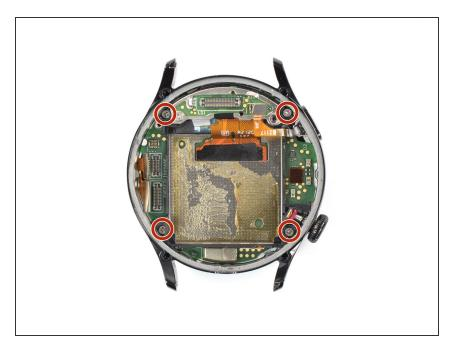
Use a Phillips screwdriver to remove the four 2.9 mm-long screws securing the motherboard.
