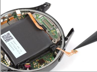
Use the tip of a spudger to disconnect the home button cable.
