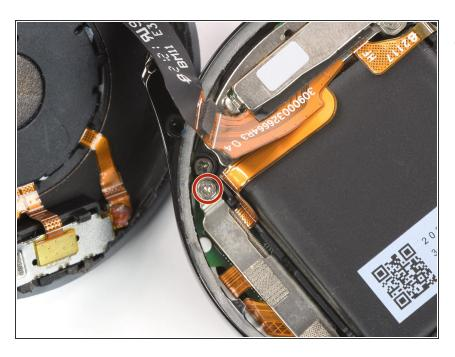
Use a Phillips screwdriver to remove the 2.9 mm-long screw from the battery bracket.
