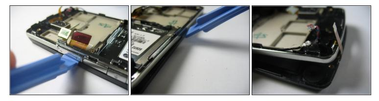
Insert a plastic opening tool below the volume rocker and gently pry the silver casing up. As
