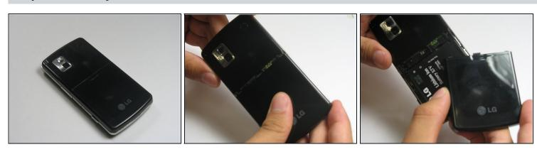
Remove the back cover by firmly pressing against the indent on the back panel. Slide the cover downward and off the phone.
