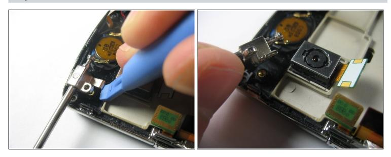
Use a plastic opening tool to carefully pry up the metal antenna guide.
