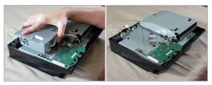
• Remove the power supply by lifting it straight up.
