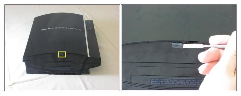
• Remove the rubber screw cover near the hard drive cover with a spudger.
