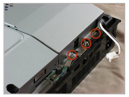
Remove the screws on the back of the power supply with a Phillips #2 screwdriver.
