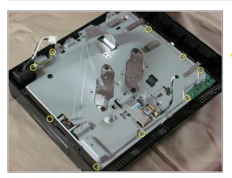
Remove nine screws (Phillips #2) from the perimeter of the metal plate covering the motherboard.
