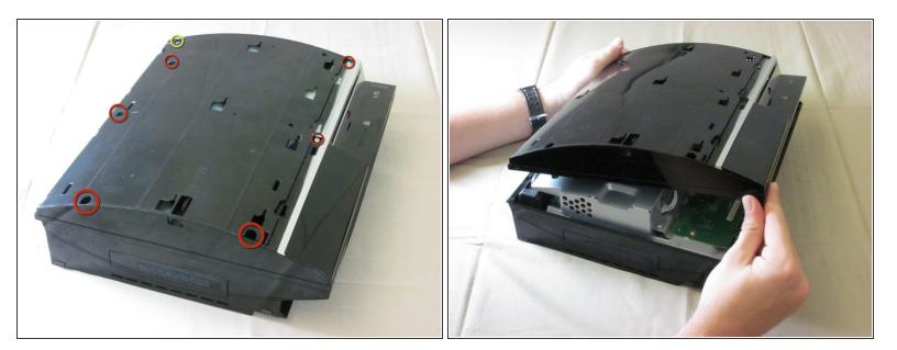
• Remove the seven screws in the top cover with a Phillips #2 screwdriver.
