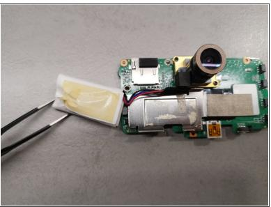
The battery is attached to the board with a small piece of tape.
