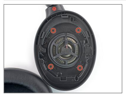
Use a Phillips screwdriver to remove the four 10.4 mm-long screws securing the plastic cover of the earcup frame.
