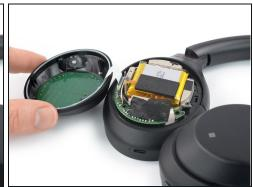
⚠ Avoid straining the gesture control cable during the following procedure.
