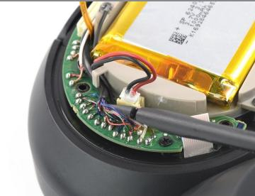
• Use the flat end of a spudger or an opening pick to carefully fold the cables blocking the battery connector to the side until you get free access to the connector.
