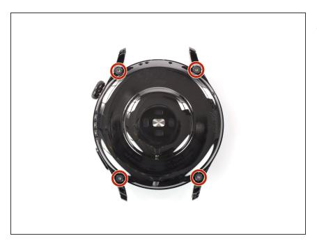
Use a Torx T3 screwdriver to remove the four 4 mm-long screws on the back of the Huawei Watch 3.
