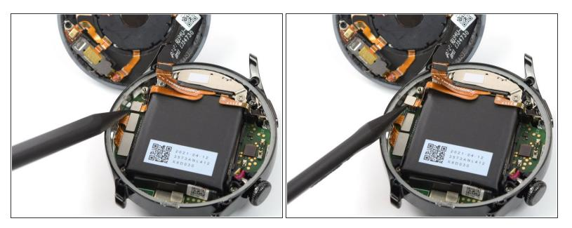
• Use the tip of a spudger to pry up and disconnect the battery connector.
