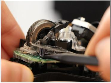
• Use your spudger to push the vertical front part of the multiswitch outwards to unhook the top part of the switch casing.
