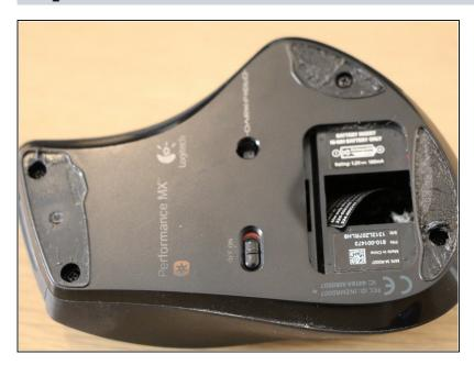
Use a 00 Phillips-Head screwdriver to remove the screws at the bottom of the mouse.
