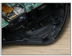
• Slide the bottom to the side while removing the top
