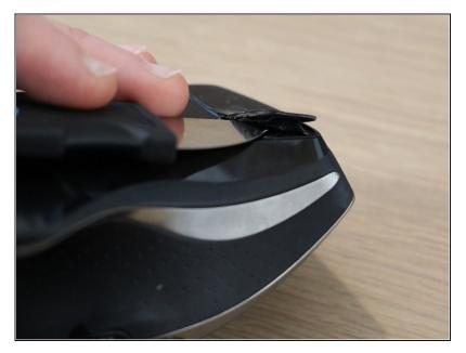
• To access the screws necessary to open the mouse, you must remove the pads on the bottom of the mouse. Use a sharp tool such as an iFixit Jimmy tool or an X-acto knife to separate the pad from the case. Each pad has two layers. Ideally, both should remain attached, but this is hard to achieve.
