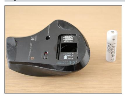
On the back of the mouse, slide the power switch so that the red area is showing to turn off the mouse. Pry open the panel on the bottom to remove the battery.
