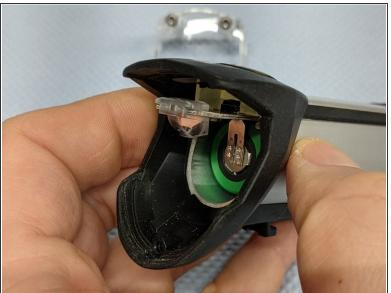
The focusing mirror is clamped behind the rubberized housing. It can be levered out of the holder with a screwdriver.
