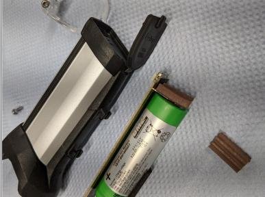
This step is optional. A little foam should be used to prevent the battery unit from moving in the housing. Follow the steps in reverse order to reassemble your device
