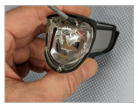
Remove the three Torx-screws.
