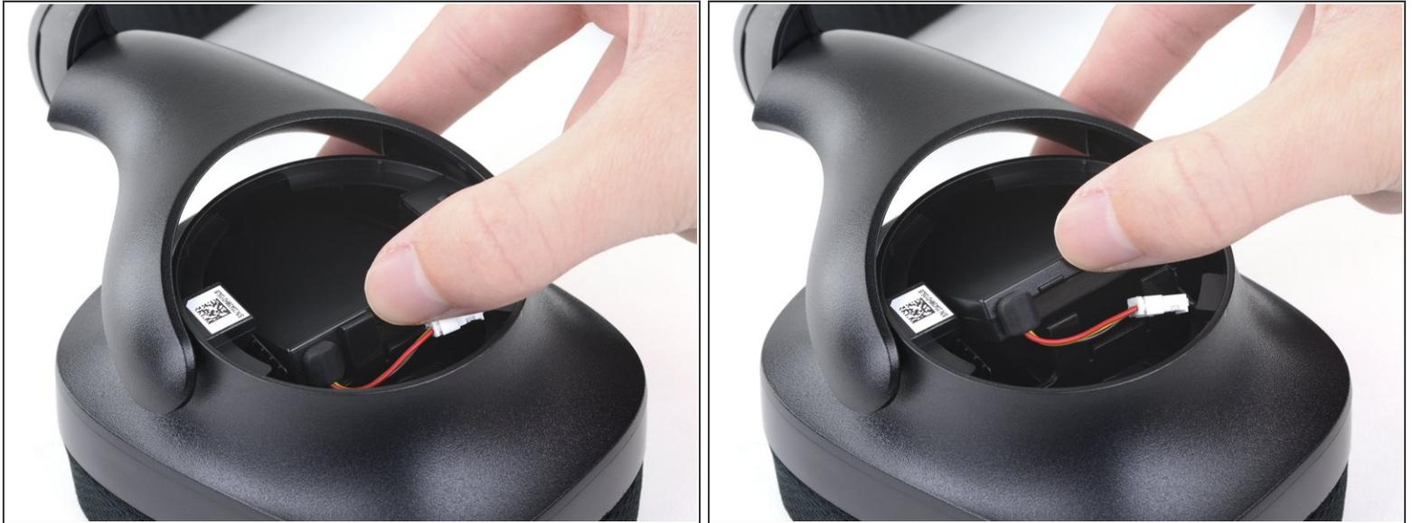
**⚠** The battery is still connected to the headset by cables at the bottom of the battery recess. Do not try to completely remove the battery before disconnecting it.
