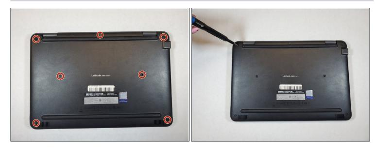
Use a Phillips #0 screwdriver to remove the seven 7 mm screws securing the back case.
