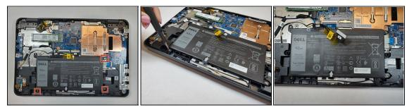
• Use a Phillips #0 screwdriver to remove the three 3 mm screws from the battery.
