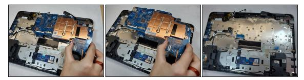
• Carefully lift the motherboard up to remove it from the computer.
