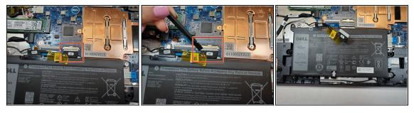
• Use a spudger to disconnect the battery cable from the motherboard located at the top of the battery.
