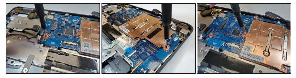
• Use the Phillips #0 screwdriver to remove the five 3 mm screws that secure the motherboard.
